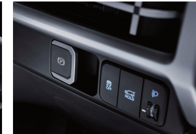
Electronic Parking Brake (EPB)
