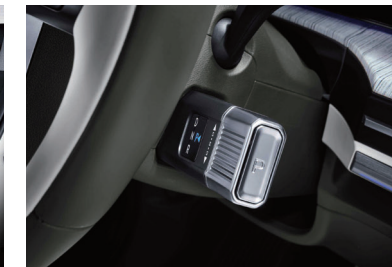
Column-type Shift by Wire (SBW)
