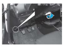
Pull the release lever to unlatch the hood. The hood should pop open slightly.
