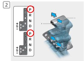
If automatic transmission: move shift lever to parking position (P)
