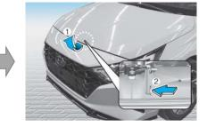
Raise the hood slightly, push the secondary latch up (1) inside of the hood center and lift the hood (2)
