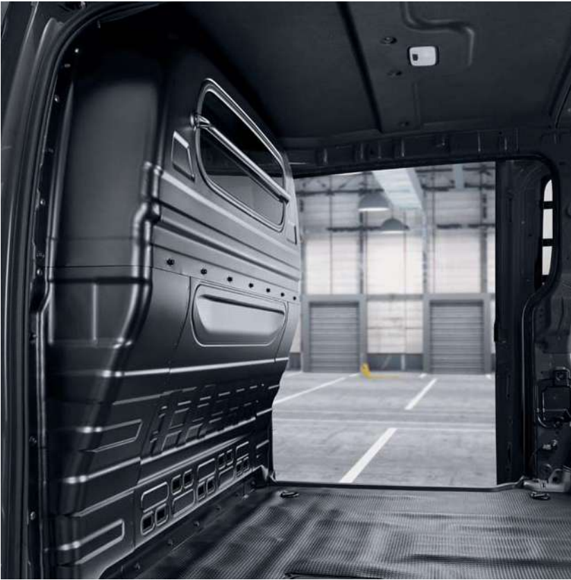
Passenger / cargo space bulkhead
