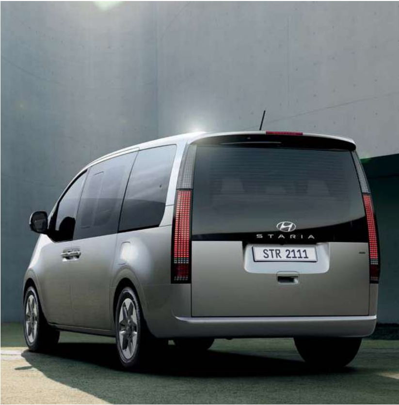
Parametric pixel lights (LED rear combination lamp)
