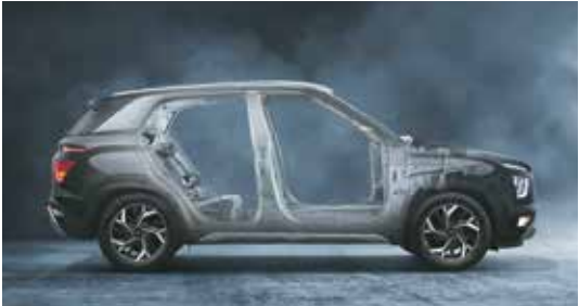
Strong body structure with AHSS
