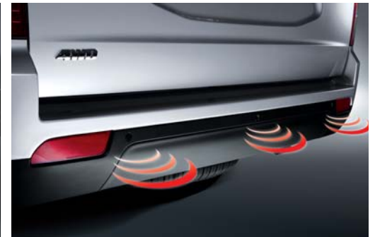
Backup warning system
