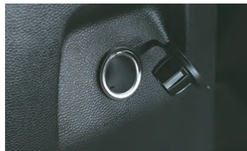
Front and Rear Power Outlets
