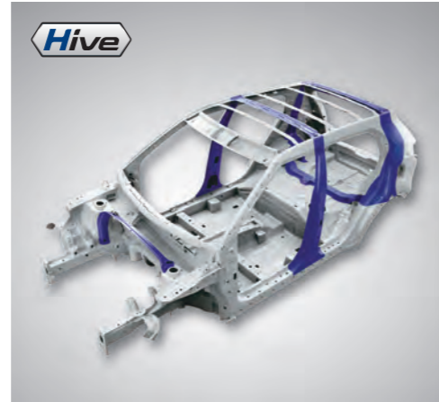
HIVE Structure Design (Engine Room, B&C Pillar) to reduce side impact and improve durability
