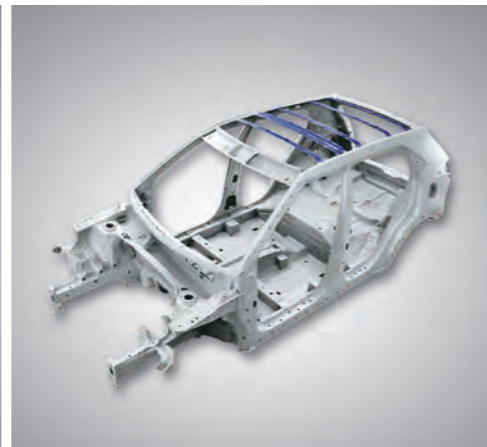
5-Bar Cross Members on Roof for enhanced roof strength
